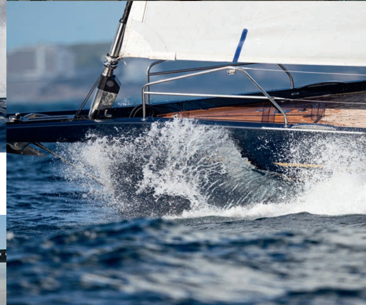
A high modulus carbon mast, carbon boom and super lightweight AEROSix carbon rigging have shaved weight off the 885GT. Her crew reported speeds up to 20 knots on their Vigo to Gibraltar passage
