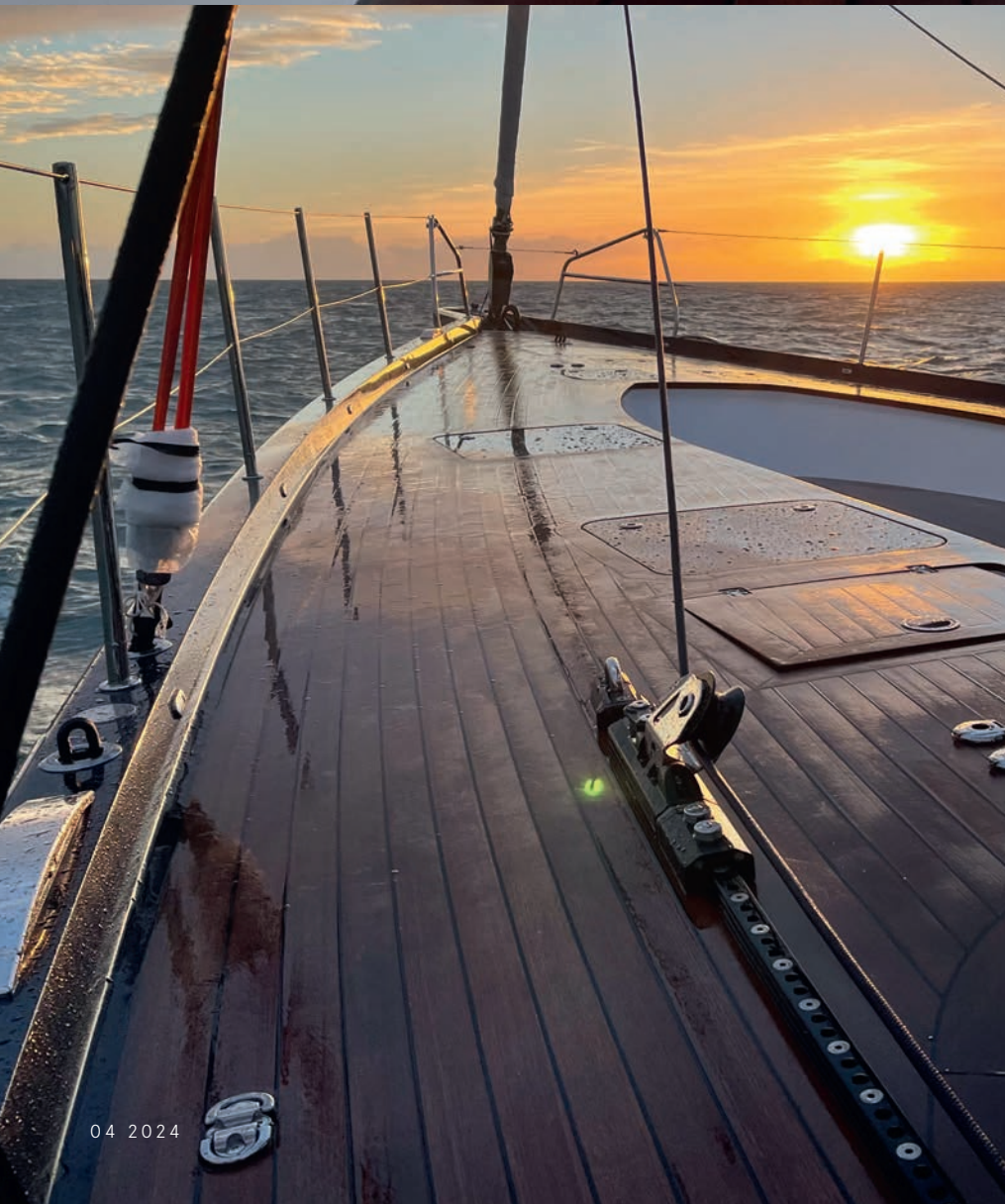
Flush padeyes and under-deck sheeting contribute to a clean deck
