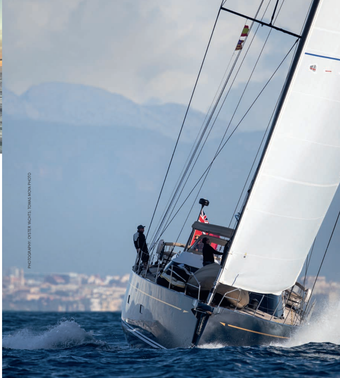
A high modulus carbon mast, carbon boom and super lightweight AEROSix carbon rigging have shaved weight off the 885GT. Her crew reported speeds up to 20 knots on their Vigo to Gibraltar passage
